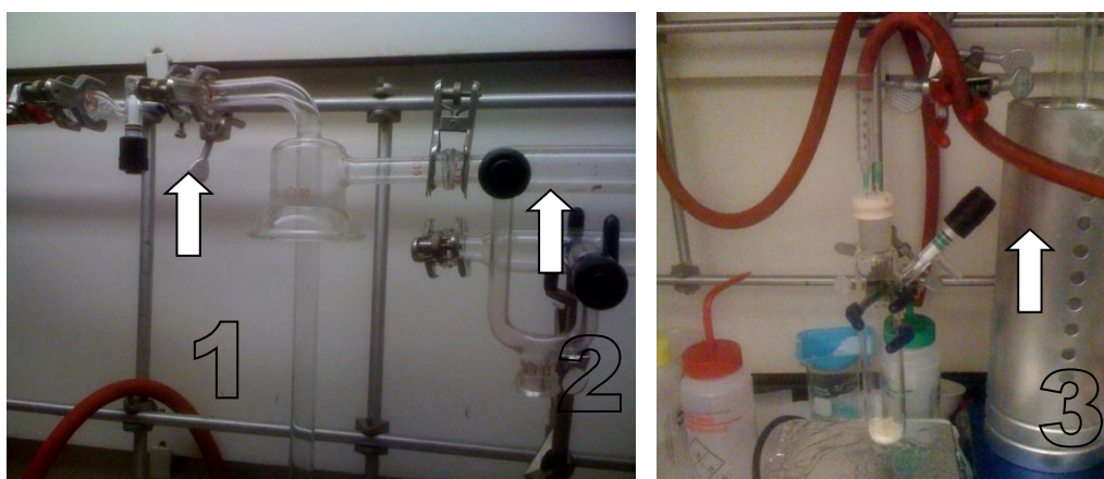
Figure B.4: Vacuum pump valves
